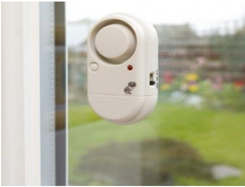
Window Shock Alarm (small alarm that is stuck to window panes that will sound an alarm if smashed or attempted to be damaged)
