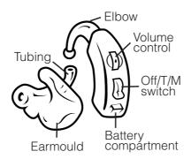
Don't unscrew the elbow (see diagram) from the hearing aid. Instead, gently pull the plastic tubing off the elbow but not from the mould. Wash the earmould and tubing in warm soapy water, and rinse them.
