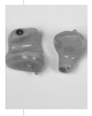
In-the-ear (ITE) and in-the-canal (ITC) aids have their working parts in the earmould so the whole aid fits into your ear. They tend to need repairing more often than BTE aids. Some ITE aids can be seen from the side. The smallest in-the-canal aids fit right inside your ear canal, where they cannot be seen. If you have severe hearing loss, or very small ear canals, these aids will probably not suit you.
